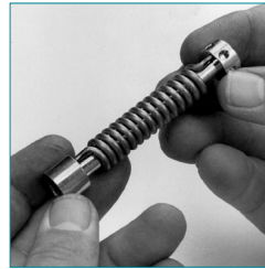
1. Assemble spring cartridge as shown.
